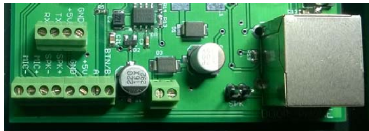
Figure 6: The 4-button outdoor unit provides both screw terminals and an RJ45 connector for interconnecting the outdoor and indoor units.
