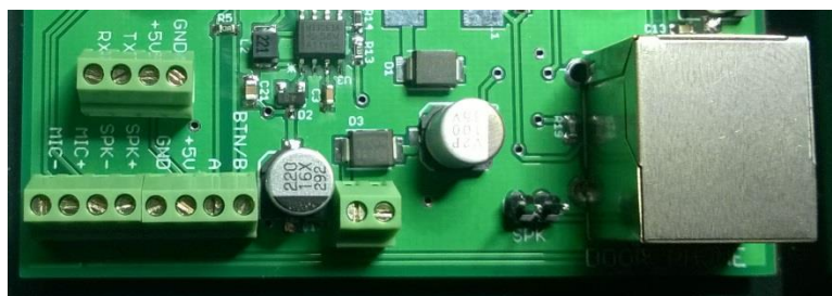
Figure 5: The 4-button outdoor unit provides both screw terminals and an RJ45 connector for interconnecting the outdoor and indoor units.
